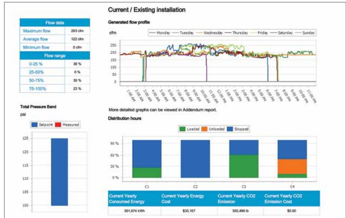
USAGE REPORT. An air audit can show you exactly the amount of air used on any given day. This data can be used to project how much energy will be used over an entire ginning season which allows for budget and planning purposes.
